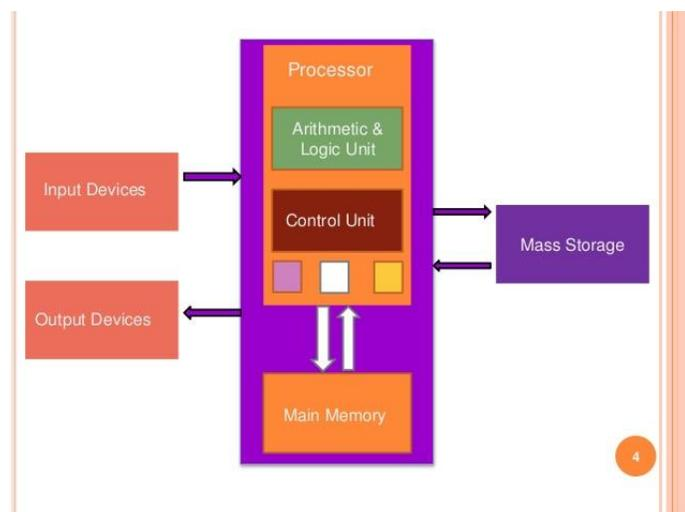
The control unit will manage the process of moving data and program into and out of memory and also deal with carrying out (executing) program instructions - one at a time. This includes the idea of a 'register' to hold intermediate values. In the illustration above, the 'accumulator' is one such register.
