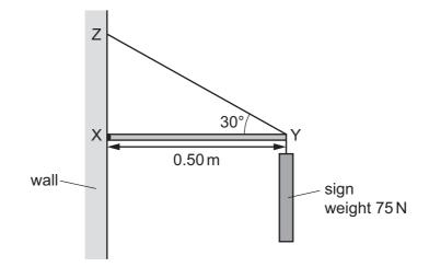
The frame consists of a horizontal rod XY and a rod YZ that is at an angle of  $30^{\circ}$  to the horizontal. Rod XY is attached to the wall by a hinge at X and has length 0.50 m. Assume that the weights of the rods are negligible.
