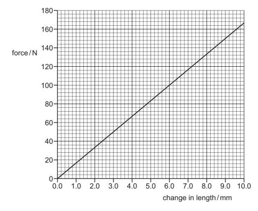
One of these springs is placed in each corner of a horizontal square plate. The axis of each spring is in a vertical direction. These four springs support a total load of 160 N.
