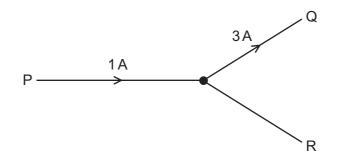
How much charge passes a given point in wire R in a time of 5 s?
