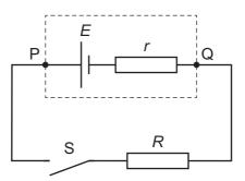
The potential difference (p.d.) between P and Q is V.
