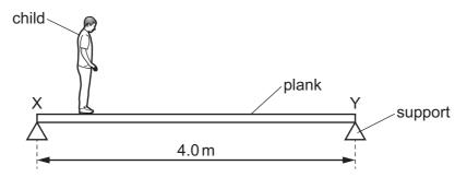
The plank rests on fixed supports at its ends X and Y.
