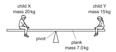
The plank has a mass of 7.0 kg and has a pivot at its midpoint. The plank is horizontal and in equilibrium.
