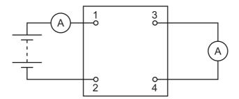
The currents in the two ammeters are identical.
