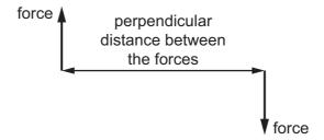
How is the torque of the couple calculated?
