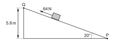
What is the work done against the frictional force acting on the block between P and Q?
