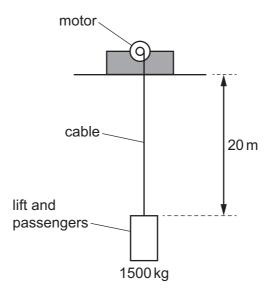
The lift and passengers have a combined mass of 1500 kg. The motor raises the lift at constant speed through a distance of 20 m.
