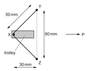
X is at the centre of the elastic and the trolley is to be propelled in the direction P at right angles to YZ. The tension in the elastic is 4.0 N.
