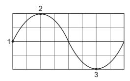
What are possible angles between the plane of the coil and the magnetic field direction at the times represented by points 1, 2 and 3?
