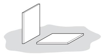
After a few hours, the vertical tile has started to sink into the soft earth. The horizontal one has **not** started to sink.
