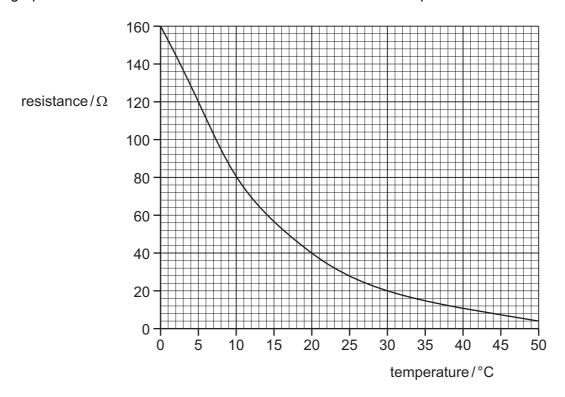
The thermistor is at a temperature of 10  $^{\circ}$ C and is connected in series with a fixed resistor of resistance 20  $\Omega$ .
