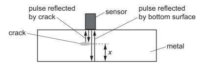
The reflection from the crack is received back at the sensor  $1.0 \times 10^{-5} \, \text{s}$  after the pulse is sent out.
