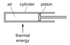
As the air inside the cylinder is heated, the piston moves to the right.
