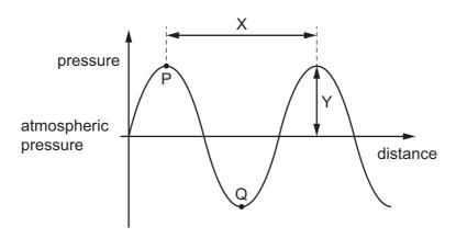
Which point on the diagram represents a rarefaction and what is the wavelength of the sound wave?
