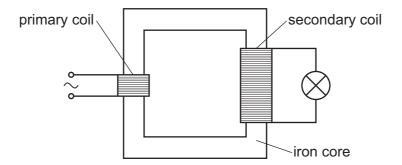
There are more turns on the secondary coil than on the primary coil.
