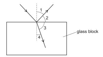
The ray of light is partially reflected back into the air and partially refracted into the glass block.
