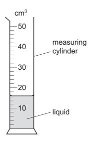
What is the volume of liquid in the measuring cylinder?
