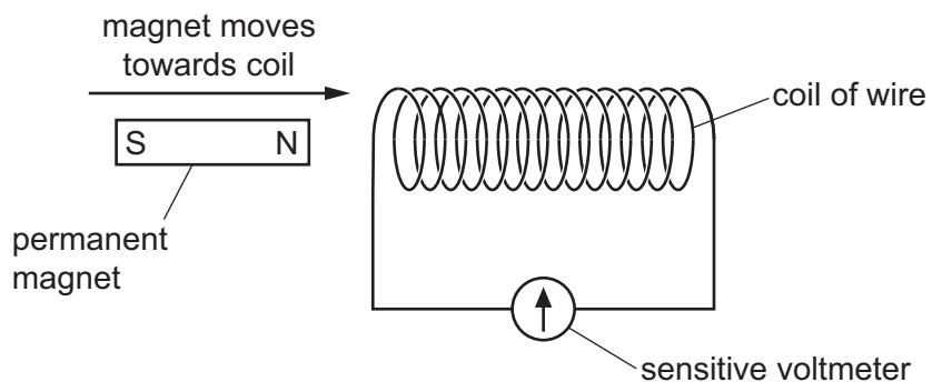
When the magnet moves towards the coil of wire, an electromotive force (e.m.f.) is induced.
