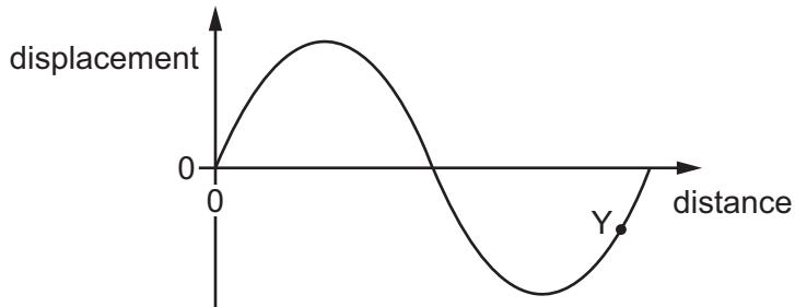
Position Y represents the displacement of a particle in the sound wave at a particular distance from the source at this instant.
