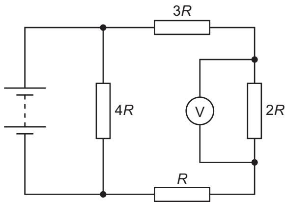
The voltmeter reading is 2 V.
