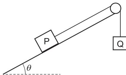
Block P moves up the slope with a constant velocity  $v$ . The slope is at angle  $\theta$  to the horizontal.
