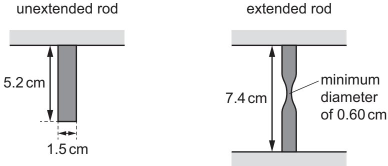
What is the maximum stress acting on the steel rod when the length is 7.4 cm?
