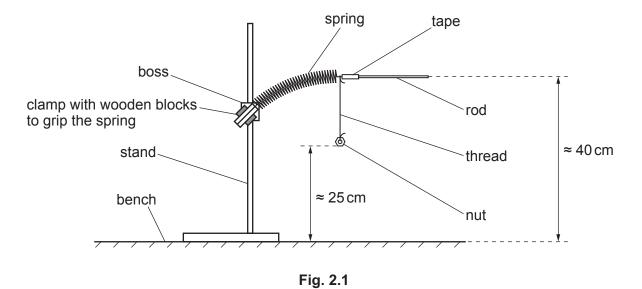
The rod should be horizontal and approximately 40 cm above the bench. The nut should be approximately 25 cm above the bench.
